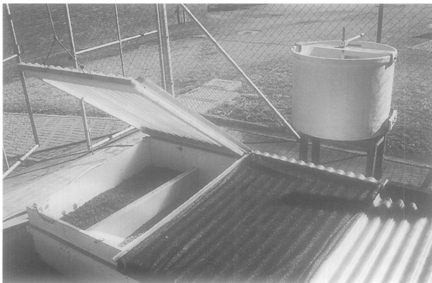
FIG. 4. CSIR outdoor sorghum malting system. Foreground – germination box. Background – steeping tank.
